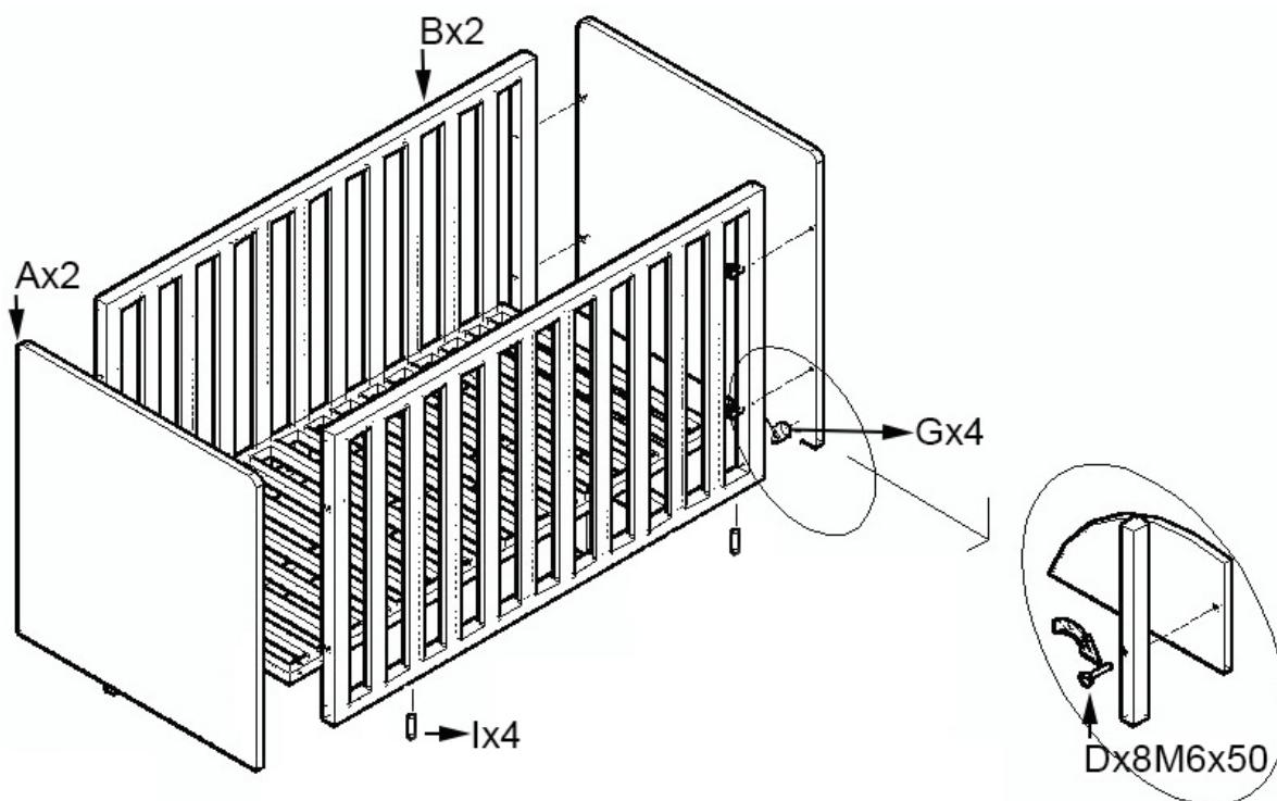
**Step 2 :** Use both end panels **A**, both sides **B**, eight bolts **D**, four eccentrics **G** and four wooden dowels **I**
