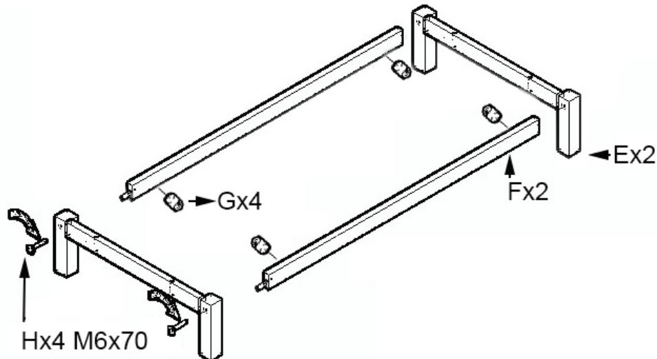
**Step 1 :** Use both crossbars **F**, both leg frames **E**, four eccentrics **G** and four connectors **H**
