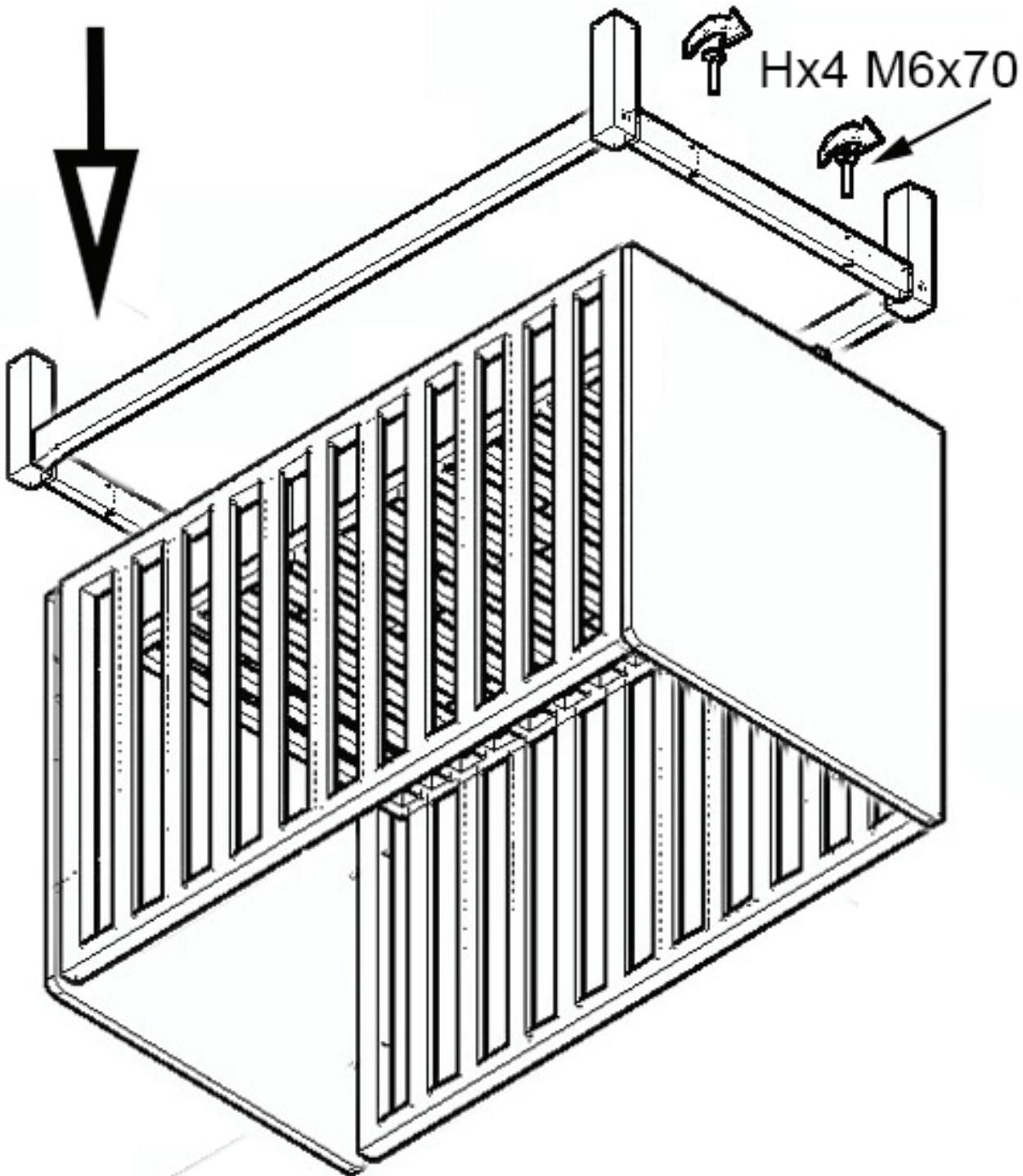
**Step 3 : Use the parts of step 1 and 2 and four connectors H**
