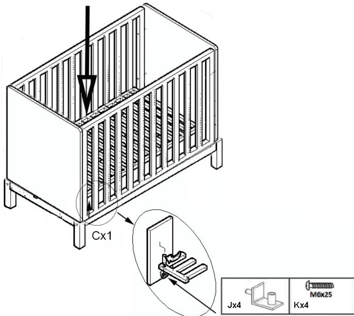
**Step 4 :** Use the parts of step 3, the slatted bottom **C**, the four bottom supports **J** and four bolts **K**
